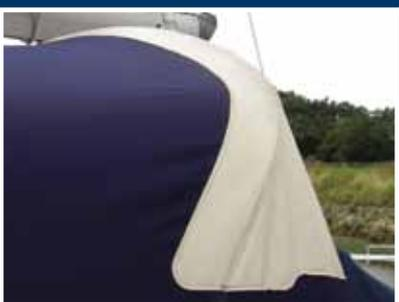
The Sacrificial Finger Strip is an alternative option, used when the C&J Marine Sprayhood Grab Handle cannot be installed. The finger strip is attached to the rear edge of the Sprayhood cover and is designed to also protect the Sprayhood from wear and chafing. The Finger Strip is available in two material options – either hardwearing, durable PVC available in a wide range of complimentary colours, or a more luxurious pearl grey leather.
