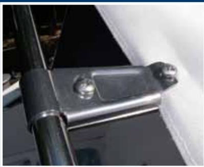
The C&J Marine Sprayhood Grab Handle standard design consists of a combination of strong nylon/stainless steel standoff and endplug fittings that are more than adequate for their intended purpose. However, for the extra quality, strength and appearance, C&J Marine offer the option of the solid stainless steel standoff and endplug fittings.
