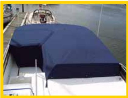
Most Flybridge Tonneau covers also need a degree of support to allow water to shed away and not collect on the cover. Stainless steel, vertical support poles are supplied with the cover. These adjustable poles support and 'peak' the cover to aid the shedding of water away.
