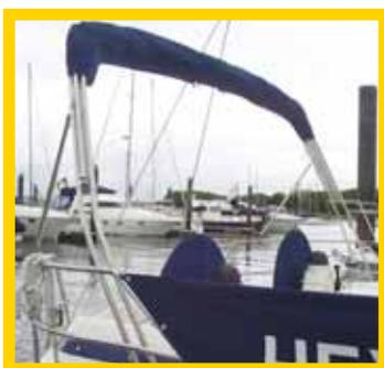
When in use the C&J Bimini is held in place aft by stainless steel support bars and tensioned forward with strong adjustable webbing straps.
