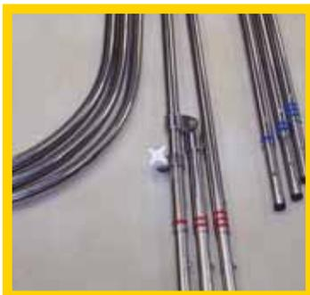
Heavy gauge, marine grade, tubular stainless steel is used in the construction of the framework. These frames are split and jointed three times, using spring loaded pins, once at the centre top and once on each vertical side, just below the radius corners. This, together with our clever colour coding system enables the frame to be stored and, when required, erected with ease.
